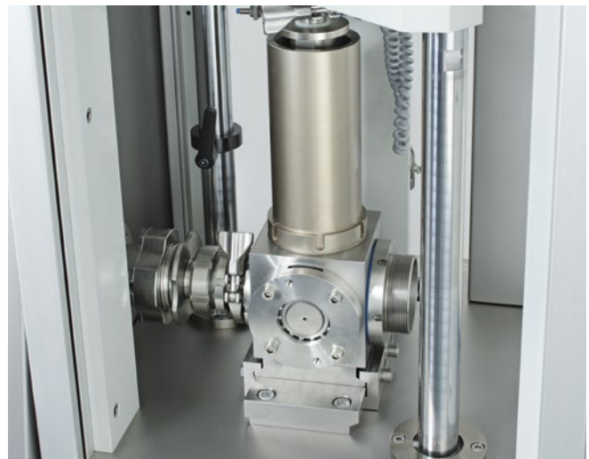
Volumetric dosing of HDP – high accuracy of filling quantity
