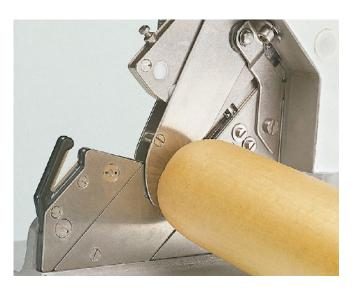
Excess casing or bag ends can be trimmed with the integrated cutoff knife.
