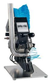
Version with pneumatic cutter and GSE (automatic looper)
