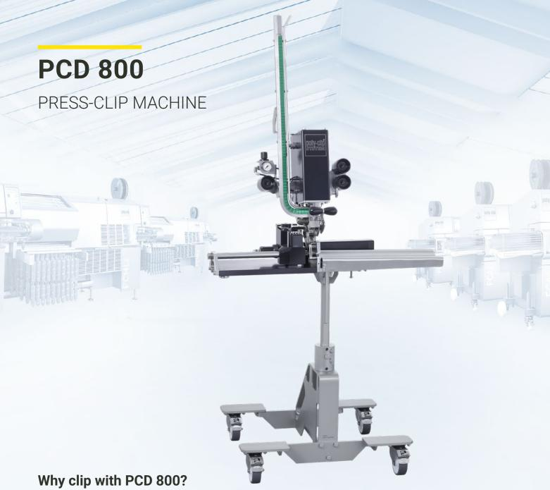
The special clipping machine PCD is suitable for closing stretch casings of different sizes. Typical products are cooked ham, smoked products, poultry meat as well as whole muscles which are to be processed afterwards. Large calibres up to 200 mm can be closed easily.
