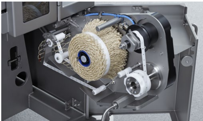
Retractable automatic looper GSA for easy reloading of loops
