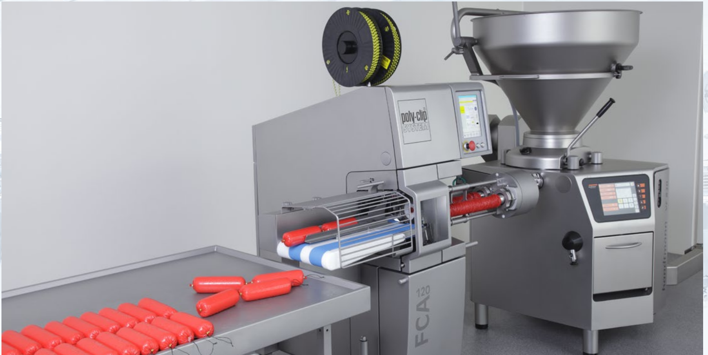
FCA 120 – the specialist machine for high speed production of calibres up to 120 mm
