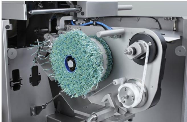
Retractable automatic looper GSA for easy reloading of loops
