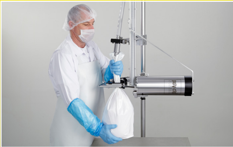
EZ 800 horizontal version with mounting bracket and vertical vacuum nozzle for heavy, bulky products
