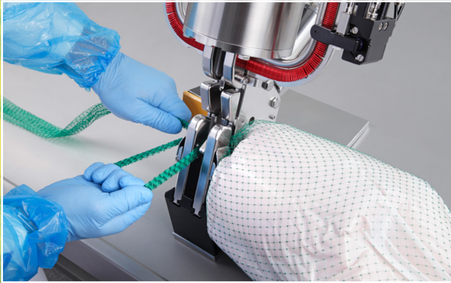
Trigger fitted on left, for formation of a loop prior to filling of the net
