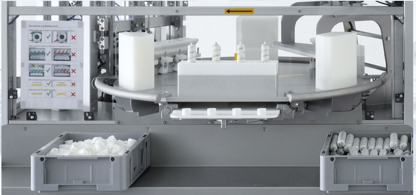
Turntable with four holders for clip-pak®
