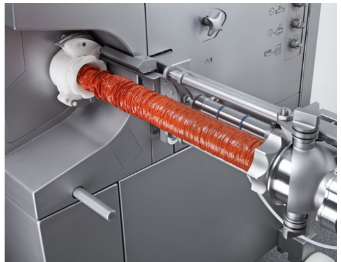
Safety casing brake with hand guard
